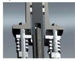
Rod-Seal<sup>®</sup> valves offer the unique Super Closure feature. A cross-head component, mounted at the end of the ram, compresses the stuffing-box gland only when the valve is fully closed. Thus, all the forces of actuation are carried by the guide bush to the packing rings and the radial seal at the top of the valve. This increased closing power ensures a tight shut-off to the process and the atmosphere. This sealing force eases when opening the valve.
