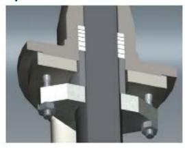
Ram-Seal<sup>®</sup> valves use packing rings for sealing to atmosphere. The packing rings are tightened using the stuffing-box gland to give a radial seal to atmosphere around the ram. Packing rings can be ordered in TVE/KEV or Graphite (suitable for high temperature or FIRE SAFE operation) or even in a mix of both. More specialized packing arrangements are available, including Chevron PTFE or Garlock graphite sealing sets.
